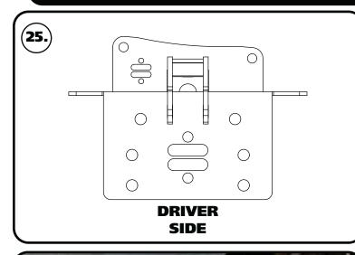
**25.** *Diagram 25* illustrates the Driver side upper control arm mount. This mount is mounted on the outside of the frame, over top the cradle The (6) holes of the upper control arm mount, align with the cradle and frame holes.
