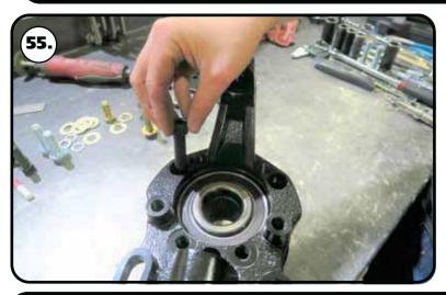
**55.** The Hub is attached to the spindle using (4) M12-1.50 x 40 SHCS. Apply RED Loctite to each of the mounting bolts. Insert them into the correct holes and Torque to 99 ftlbs.
