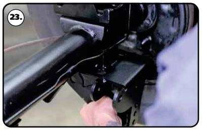
**23.** The kit includes a Driver and Passenger lower axle mount; the two are different. The Passenger mount has the panhard bar mount built into it. **Image 23** shows the Passenger mount. Hold the mount up in place against the bottom of the axle tube. The tabs will nest against the bottom of the leaf spring pad.
