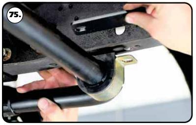
**73.** Open the sway bar bushing at the split and slip it onto the sway bar. Do this for both bushings.
