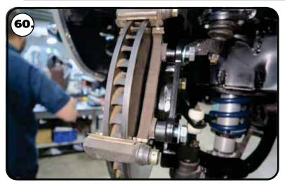
**60.** The OEM caliper bracket will bolt to the spindle mount. Install a M12 flat washer on each of (2) M12-1.75 x 30mm hex bolts. Insert the bolts through the caliper bracket. Line the caliper mount up with the hardware and thread in the bolts.
