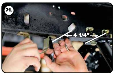
**71.** Use a tape measure to put a mark on the frame **4 1/4**" from the front edge of the cradle mount. Align the back edge of the sway bar mounting strap with the mark on the frame. Hold the mounting strap in the center of the frame and mark the center of each mounting hole. The mounting holes need to be marked on each frame rail.
