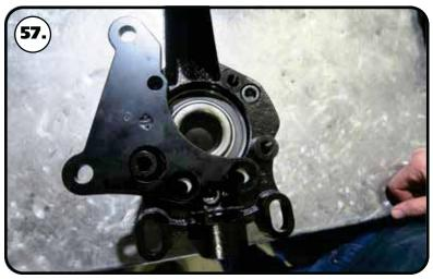
**57** The caliper brackets are side specific. They have a D & P stamped in them. Lay the correct side caliper bracket on top of the shims, aligning the mounting holes with the mounting holes of the bracket. The counter sunk holes should facing up.
