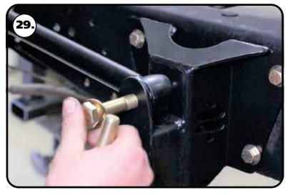
**29.** Line the through hole of the R-Joint with the of holes of the frame mount. Install a 5/8" flat washer on to a 5/8"-18 x 3 1/2" hex bolt, insert into the lined up holes. Install a 5/8" flat washer followed by a 5/8"-18 nylok nut. Repeat on both sides and tighten the bolts/nuts enough to eliminate any gaps.
