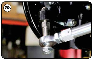
**70.** Install a 1/8" thick aluminum on the bottom side of the heim end followed by a 5/8"-18 thin nylok nut on the stud. Torque the nut to 45 ft-lbs.
