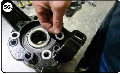
**56.** Lay a .062" thick, 1/2" ID shim on each of the caliper brackets (3) mounting holes.
