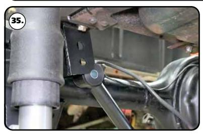
**35.** Remove the bolt that attaches the brake hose to the bracket. This will allow you to move the brake line out of the way to cut the bracket off the axle tube.
