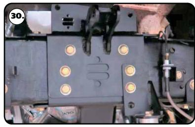
**28.** Install a 7/16" flat washer on a 7/16"-14 x 1 3/4" hex bolt. Insert the bolt in the top hole of the rear (3) bolt holes. This bolt will go through the upper control arm mount, cradle plate, & engine mount. Install a 7/16" flat washer and 7/16"-14 nylok nut on the threads of the bolt. DO NOT INSTALL A BOLT IN THE LOWER HOLE OF THE ENGINE MOUNT HOLE AT THIS TIME.
