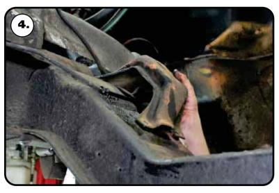
**4.** Remove the OEM engine mount stands.
