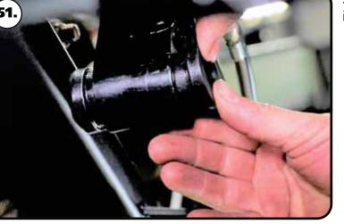
**51.** Insert the 2nd half of the rack bushings into the rack. Do this for each mount.
