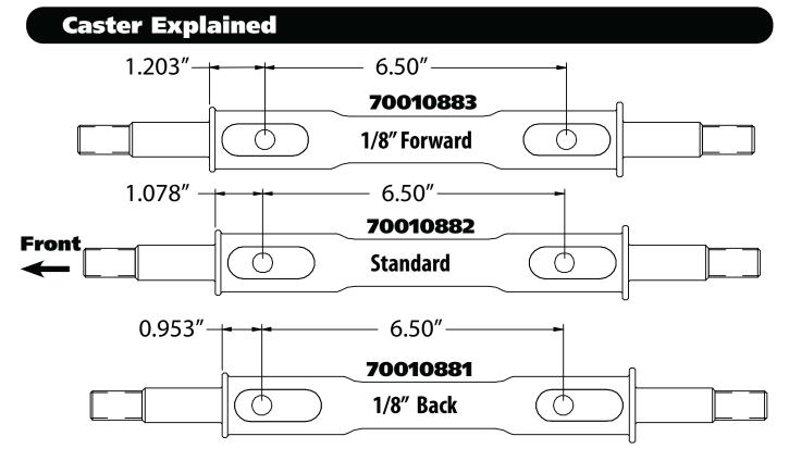
These StrongArms come equipped with a changeable caster slug setup. This allows you to add or remove caster from the front suspension, if desired. The caster slugs that come supplied in the kit are standard (70010882). The caster slugs allow you to add or remove caster without having to use a stack of shims. If more or less caster is desired, optional slugs can be purchased from Ridetech or your Ridetech dealer.
