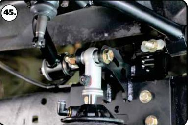
**45.** Install a 1/2" flat washer on a 1/2"-13 x 3" hex bolt. Insert the bolt/washer into the mount/shock. Install a 1/2" flat washer & 1/2"-13 nylok nut. Torque the hardware to 75 ft-lbs.
