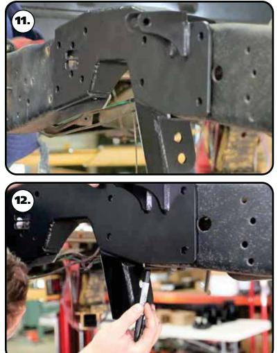
**11.** After cutting, slip the c-notch over the frame to check the fitment. The cut areas of the frame may require grinding for the c-notch to fit.
