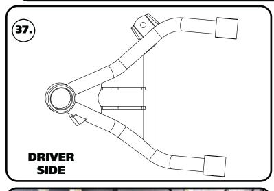
**37.** The lower control arms are marked "D" for Driver and "P" for Passenger. The ball joint pin points up and the sway bar mount is on the front side of the arm. **Diagram 37** shows a top view of the Driver lower control arm.
