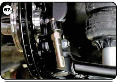
**67.** Install the stud with the hex into the steering arm with the taper going into the steering arm. Install the 7/16"-20 castle nut onto the tie rod stud. Torque the nuts to 35 ftlbs and tighten as needed to align cotter pin hole and install cotter pin.
