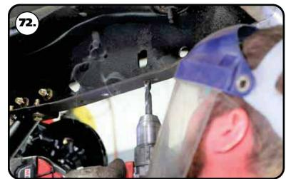
**72.** Drill the holes using a 3/8" drill bit.
