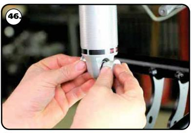
**46.** Insert the shock bearing t-bushings into the bearing of the shock body. The small outside diameter of the t-bushing will insert into the shock bearing.
