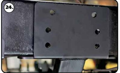
**24.** Position the cradle so that the (6) holes of the side plate align with the rivet holes in the frame.
