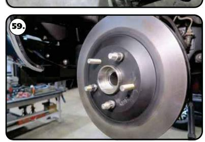
**59.** Install the rotor on the hub. Thread some lug nuts on the threads of the hub to hold the rotor tight on the hub.
