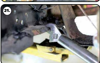
**21.** We used an adjustable wrench to bend the flange flat. Tighten the adjustable wrench tight to the rail and use the wrench to bend it upward. You will need to work up and down the frame rail bending it up to get the frame rail flat.
