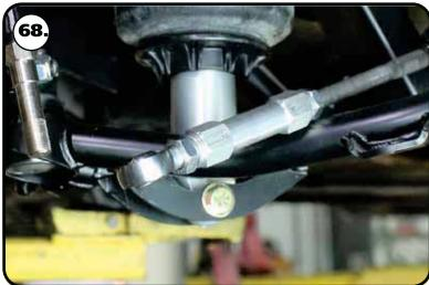
**68.** The tie rod adjusters have (2) different thread sizes, 5/8"-18 LH & 9/16"-18. The left hand threaded heim will thread into the 5/8"-18 end. The rack threads into the 9/16"-18 end. Install the 5/8"-18 LH jam nut on the heim end. Install a 9/16"-18 jam nut on the threads of the rack. Thread the heim into the adjuster and thread the adjuster onto the rack.
