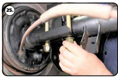
**25.** Hold the mount in place and install a 5/8" flat washer and 5/8"-18 nylok nut on the threads of the u-bolts sticking through the axle mount. Tighten the nuts evenly in a criss-cross fashion making sure the tabs of the axle mount are touching the leaf spring pad evenly. Torque the nuts in a criss-cross fashion to 75 ftlbs. Repeat on the other side.
