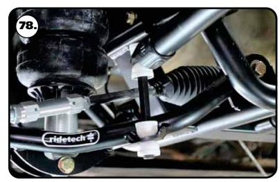
**78.** Tighten the end link barrel nut until it is flush with the end of the bolt, and then tighten it 2-3 more complete rounds. Torque the frame bolts to 45 ft-lbs.
