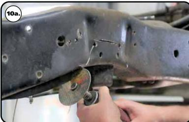
**10a & 10b.** Cut the notch with a saw-z-all, cutoff wheel, or plasma cutter. Grind all edges smooth. Cut the sides of the frame and across the bottom of the rail. The cuts on the bottom of the frame rail will be parallel with each other. The side frame cuts will blend into the drilled holes. The section of frame will fall out when cutting is complete.
