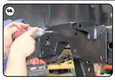
**14.** Reinstall the c-notch. The c-notch will be used as a template to drill the remaining mounting holes. Use a 7/16" Drill bit to drill the holes in the side of the frame. There are 8 holes in the side that need to be drilled.
