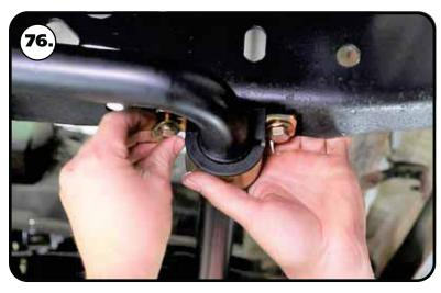
**76.** Install a 3/8" flat washer on each of (4) 3/8"-16 x 1 1/4" hex bolts. Hold the sway bar in place and insert a bolt in the mounting hole of the mounting strap. Install a 3/8" flat washer & 3/8"-16 nylok nut on the threads of the bolt. Repeat this on remaining mounting holes. Do NOT tighten the mounting bolts at this time. They need to left loose until the sway bar linkage has been attached to the lower control arm.
