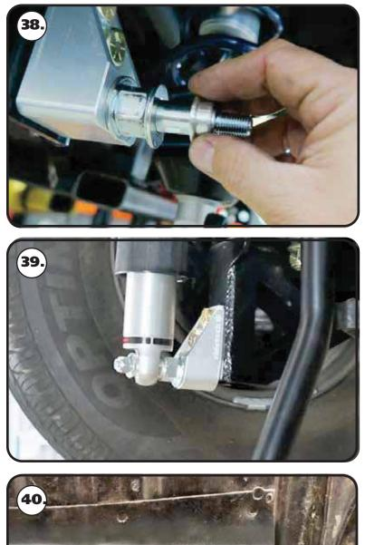
**38.** The Shock Stud requires spacers that are .400" long (90002067). Install a 5/8" ID 90002067 spacer **(Small side towards shock body)** onto the lower Shock Stud. Slide the bottom of the Shock onto the Stud. Install a second 5/8" ID 90002067 Spacer onto the Stud **(small side towards shock)**. You may need to jack the rear end up to Slide the Shock onto the Stud.
