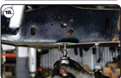
**16.** The inside of the frame rails need to be ground smooth.
