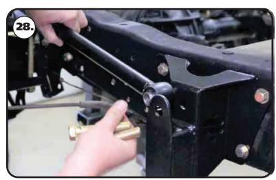
**28.** Insert (2) .625" ID x .740" long R-Joint spacers into the R-Joint of one end of each 23 3/8" center to center upper bar. The small diameter of the spacer goes into the R-joint. Insert the front of the upper bar R-Joint into the front mount. The front mount has 2 bar mounting locations. The 23 3/8" upper bar needs to be installed into the top position.
