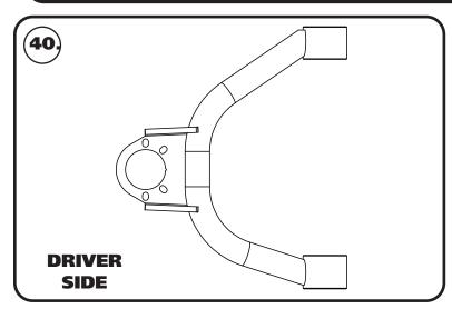
**40.** The upper control arms are marked "D" for Driver and "P" for Passenger. The ball joint pin points down and the ball joint is to the rear of the truck. **Diagram 40** shows a top view of the Driver upper control arm.
