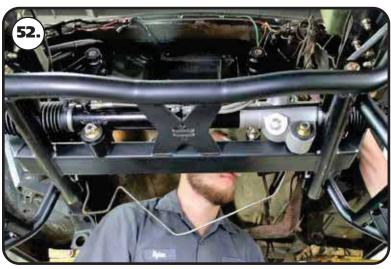
**52.** Install a M12 flat washer on a M12-1.75 x 170mm hex bolt. Insert the bolt/washer into the rack mount. Install a 1M12 flat washer & M12-1.75 nylok nut. Torque the hardware to 93 ft-lbs.
