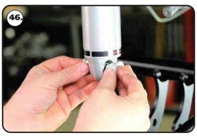
**46.** Insert the shock bearing t-bushings into the bearing of the shock body. The small outside diameter of the t-bushing will insert into the
