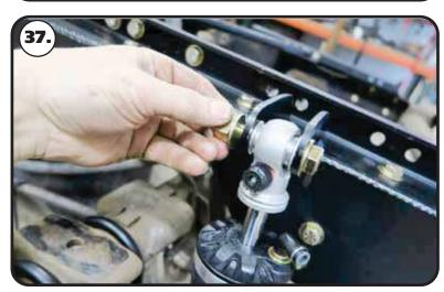
**37.** Insert the 1/2" ID Shock Bearing Spacers into the Bearing of the ShockWave/CoilOver. Install a 1/2" Flat Washer on a 1/2"-13 x 2 3/4" Bolts. Insert the top of the shock into the shock mount on the c-notch with the adjusting knob to the outside. Line up the holes and insert the bolt/washer. Install a 1/2" Flat Washer and 1/2"-13 Nylok Nut on the threads and tighten to 50 ftlbs.
