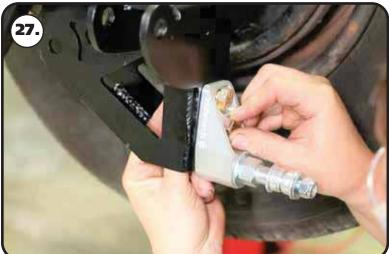
**27.** Insert the bolts through the axle mount and install the flat washers & nylok nuts on the threads sticking through. Repeat on both sides and torque the bolts/nuts to 75 ftlbs. Install a 5/8" flat washer onto the 5/8"-18 threads of the shock stud. Apply Red Loctite to the 5/8" threads of the stud. Thread the shock stud into the threaded hole of the lower mount. Repeat on both sides and torque the shock stud to 65-75 ftlbs.
