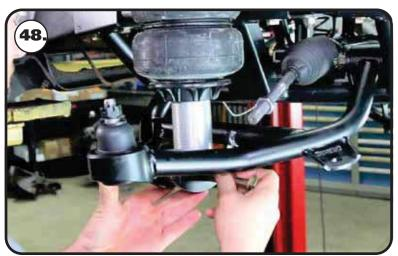
**48.** Install a 1/2" flat washer on a 1/2"-13 x 3" hex bolt. Insert the bolt/washer into the mount/shock. Install a 1/2" flat washer & 1/2"-13 nylok nut. Torque the hardware to 75 ft-lbs.
