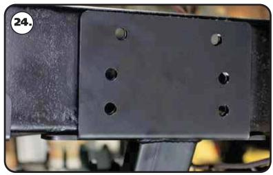
**24.** Position the cradle so that the (6) holes of the side plate align with the rivet holes in the frame.
