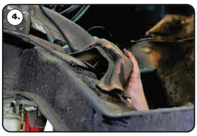
**4.** Remove the OEM engine mount stands.
