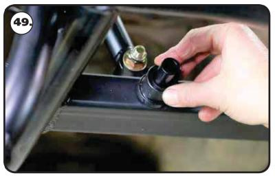
**49.** Install one half of a poly rack bushing on the rack mounting bung of the cradle. The bushing needs to be installed on the bung with the large diameter against the cradle. Install a bushing on each mounting bung.
