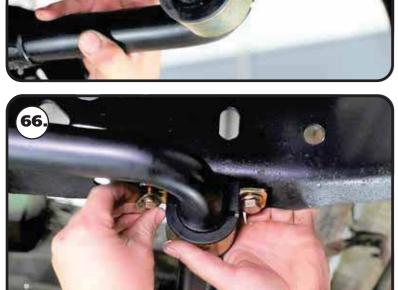
**66.** Install a 3/8" flat washer on each of (4) 3/8"-16 x 1 1/4" hex bolts. Hold the sway bar in place and insert a bolt in the mounting hole of the mounting strap. Install a 3/8" flat washer & 3/8"-16 nylok nut on the threads of the bolt. Repeat this on remaining mounting holes. Do NOT tighten the mounting bolts at this time. They need to left loose until the sway bar linkage has been attached to the lower control arm.
