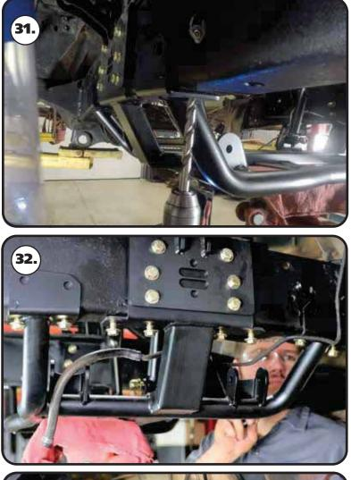
**31.** There are (8) mounting holes in the bottom mounts of each side of the cradle. All but (2) of these will need to be drilled with a 7/16" drill bit. (2) of the holes will align with factory holes.
