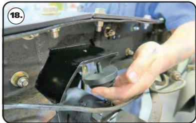
**18.** Install the bump stop using a 3/8"-16 x 1" socket head bolt, 3/8" flat washer, & 3/8"-16 nylok nut. Hold the bump stop with your hand and insert the bolt through the center of the bump stop. Line up the bolt of the bump with the drilled hole of the frame. Install a 3/8" flat washer and 3/8" nut on the threads of the bolt. Tighten to 60 in-lbs
