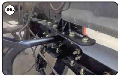
**36.** Install a 7/16" flat washer on each of (4) 7/16"-14 x 1 /4" hex bolts. Insert a bolt/washer in each top (4) holes. Install a 7/16" flat washer and 7/16"-14 nylok nut on the threads of the bolts. Torque all 7/16" cradle hardware to 70 ft-lbs. Torque the 1/2" engine mount hardware to 75 ft-lbs.
