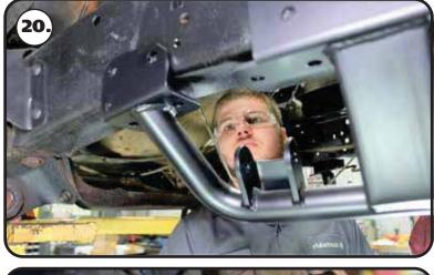
**20.** The 73-79 F100 trucks passenger frame rail has a section of the frame bent downward. This bent down area is in the location of the rear crossmember mount. This area needs to be flattened for cradle installation. The cradle can be lifted in position to mark the area that needs flattened.
