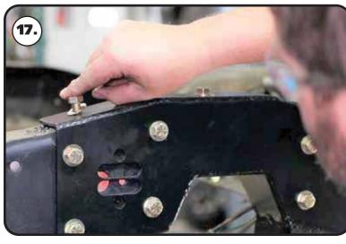
**17.** Install a 7/16" flat washer on each of (5) 7/16" x 1 1/4" bolts. This hardware gets installed in the top & bottom of the c-notch. Install a 7/16" flat washer and 7/16" nylok nut on each bolt sticking through the frame. Tighten the c-notch mounting hardware to 70 ft-lbs.
