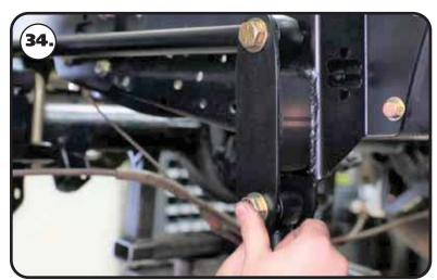
**34.** Line the through hole of the R-Joint with the of holes of the front frame mount. Install a 5/8" flat washer on to a 5/8"-18 x 3 1/2" hex bolt, insert into the lined up holes. Install a 5/8" flat washer followed by a 5/8"-18 nylok nut. Repeat on both sides and tighten the bolts/nuts enough to eliminate any gaps.
