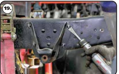
**19.** The OEM front leaf spring mounts will need to be removed from the frame rail. This can be done by either drilling the rivets out or removing the rivet heads and driving them out. We remove the rivet heads by cutting a "+" in the head with a die grinder then we cut the head off with a hammer and chisel or with an air chisel.
