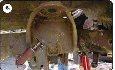
6. The OEM upper coil spring and I-beam mounts need be removed from the frame rail. This can be done by either drilling the rivets out or removing the rivet heads and driving them out. We remove the rivet heads by cutting a " + " in the head with a die grinder then we cut the head off with a hammer and chisel or with an air chisel. Once the head is removed, the rivet can be driven out with a hammer and punch.
