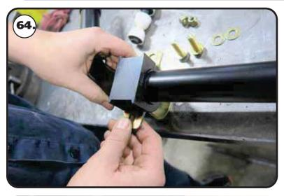
**64.** Install the bushing mounting strap on the sway bar bushing.
