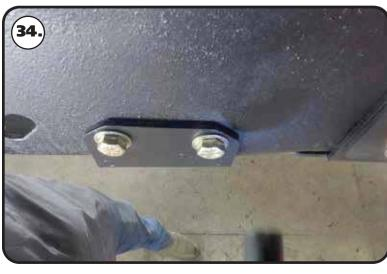
**34.** Install a 7/16" flat washer on each of (4) 7/16"-14 x 1/4" hex bolts. Insert a bolt/washer in each of the (4) holes. Install a 7/16" flat washer and 7/16"-14 nylok nut on the threads of the bolts. Again, snug the hardware down, but do not torque the hardware at this time. Do this for both sides.
