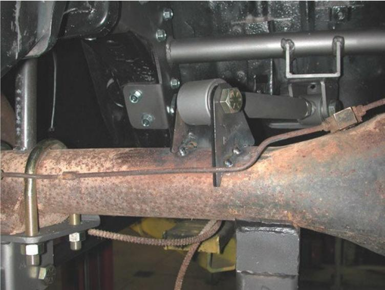
15. Check the length of the upper bar; it should be 10" C-C.
