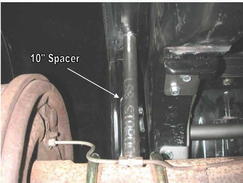
10. Raise the axle to ride height. This can be determined by measuring 10" from the top of the axle up to the body, just outside the rail.
