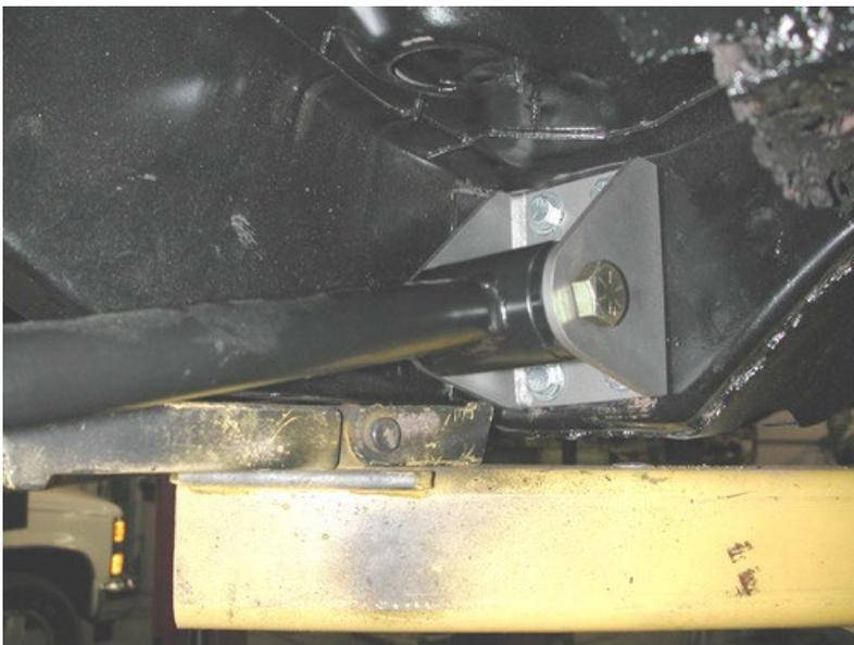
8. Bolt the new lower bar frame mount to the body using 3/8" x 1 1/4" bolts, Nylok nuts and flat washers.
