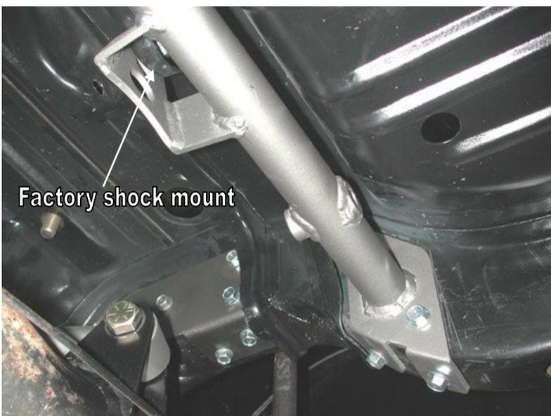
5. The upper Shockwave bridge will slide between the frame rails directly behind the factory shock cross member. The bridge will be positioned by bolting the tabs to the factory shock hole. Fasten the bridge to the factory shock mount using 1/2" x 1 1/2" bolt, flat washer and Nylok nuts. Using the bridge as a template drill the holes in the frame with a 5/16" bit. 3/8" x 1" thread forming bolts and flat washers will hold the bridge in place.
