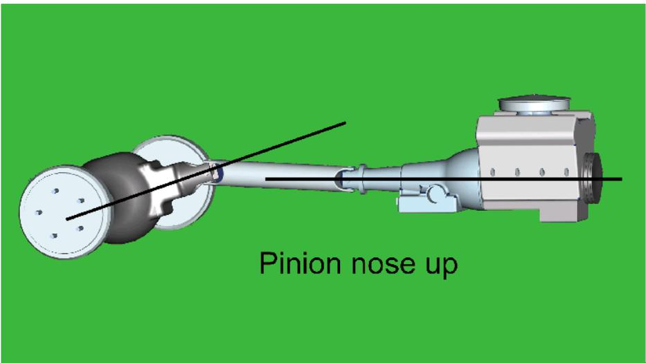
14. How do you set the pinion angle? On a single-piece shaft you want to set it up where a line drawn through the center of the engine crankshaft or output shaft of the transmission and a line drawn through the center of the pinion are parallel to each other but not the same line.
