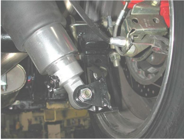
7. Bolt the lower axle bracket to the leaf spring pad using the 9/16" U-bolts and hardware supplied. Bolt the lower Shockwave mount to the axle bracket using the 1/2" x 1 1/4" bolts and Nylok nut.
