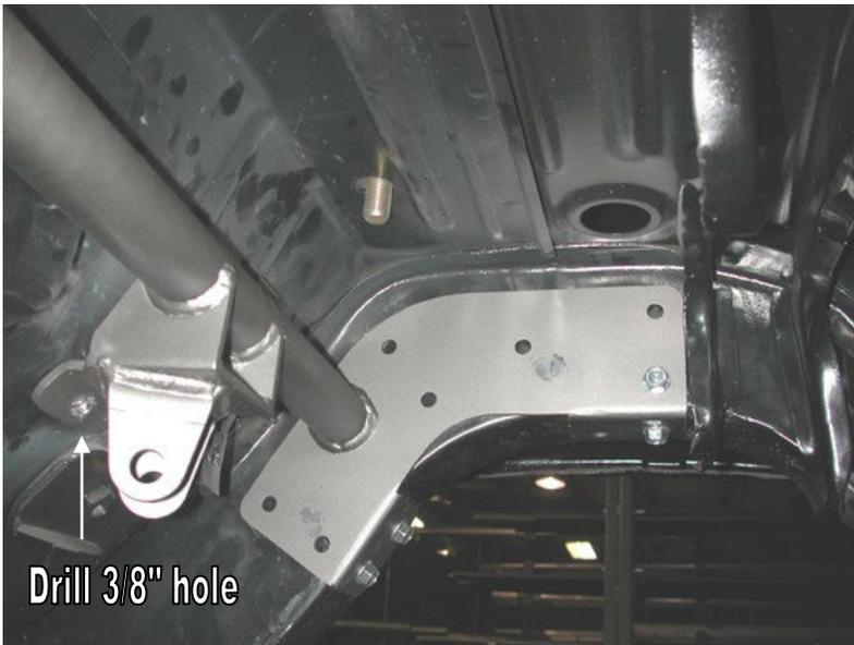
3. Slide the upper bar bridge between the frame rails. Using the bridge as a template, mark all the holes in the frame and drill with a 5/16" bit. Then secure the bridge using the 3/8" x 1" thread forming bolts and flat washers.
