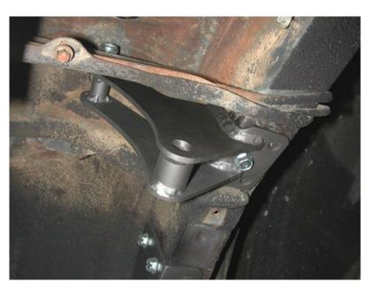
14. Attach the upper Shockwave mount to the factory upper shock mount using a ½" x 2 ¾" bolt, Nyloc nut, and flat washers. Swing the bracket out to the frame rail to mark and drill 5 holes in the frame with a 5/16" bit. Fasten with 3/8" x 1" thread forming bolts and flat washers.
