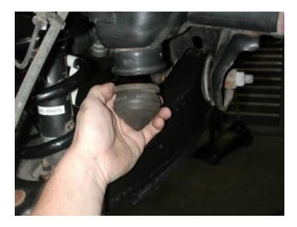
3. Remove the factory bump stop from the frame. The bump stop housing does not need to be removed.
