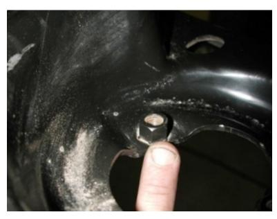
6. The factory shock was held in place with these nuts on the lower control arm. They must be removed before installing the Shockwaves. A hammer and chisel will do the job.
