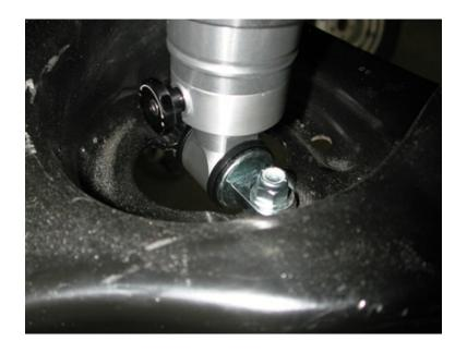
9. The bottom of the Shockwave has a T-bar installed through it. It will bolt to the **top** of the lower control arm and is secured with two 3/8" x 1 ½" bolts, two Nylok nuts and four flat washers. The reinforcement plate is to be installed between the T-Bar and the lower arm.
