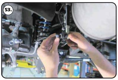
**53.** Install a M10 flat washer on the threaded stud of the lower linkage. Insert the threaded stud in the OEM sway bar. Install a M10 flat washer & on the threaded stud sticking through the sway bar. Torque the sway bar mounting and end link hardware to 37 ft-lbs.
