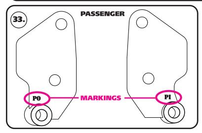
**33. Image 33** illustrates the passenger side relocation brackets. They are marked PO for Passenger Outer and PI for Passenger Inner. The flat side of the bracket is positioned to the front of the truck.
