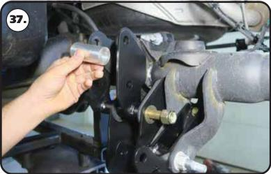
**37.** Install the 2 5/8" long spacers between the OEM upper bar mounts. Align the hole with the holes of the upper bar mounts. The top hole of the upper bar relocation brackets need to be aligned too.
