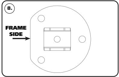
**8. Image 8** illustrates the upper coil over mount. The flat side of the mount will need to be positioned to the frame.
