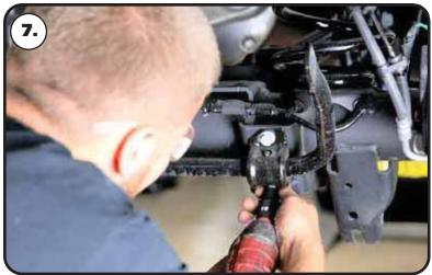
**7.** Remove the rear sway bar. It will be reinstalled after the lowering kit is installed.
