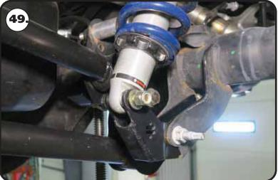
**49.** Install a 1/2" flat washer on a 1/2"-13 x 2 3/4" bolt. Insert the bolt/washer into the lower mount/shock. Install a 1/2" flat washer and 1/2"-13 nylok nut and Torque to 75 ftlbs.
