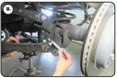
**8.** Lower the axle as far as the OEM bar bushing will allow it to go, but make sure the axle is still supported by the jack. Remove the control arm control arm bolts at the axle.
