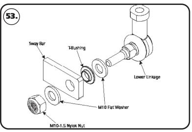
53. Install a M10 flat washer on the threaded stud of the lower linkage, followed by the T-Bushing. The small end of the T-Bushing fits into the sway bar mounting hole (See Image 53). Insert the threaded stud in the OEM sway bar. Install a M10 flat washer & M10-1.5 Nylok Nut on the threaded stud sticking through the sway bar. Torque the sway bar mounting and end link hardware to 37 ft-lbs.
