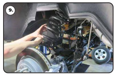
**9.** Remove the rear coil springs. You may have to push down on the end of the axle to get the coil spring out of the mount.
