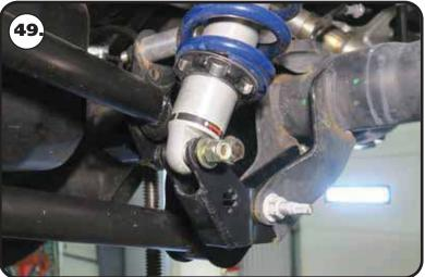
**49.** Install a 1/2" flat washer on a 1/2"-13 x 2 3/4" bolt. Insert the bolt/washer into the lower mount/shock. Install a 1/2" flat washer and 1/2"-13 nylok nut and Torque to 75 ftlbs.
