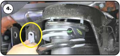
**4.** Unbolt the brake line from the frame, but retain the OEM hardware. This allows the lower control arm to move easier during the CoilOver installation.
