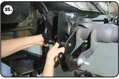
**35.** Align the sleeve of the Outer bracket with the bolt holes of the OEM lower bar mount. Push the M16-2.0 x 170mm bolt through the bracket.
