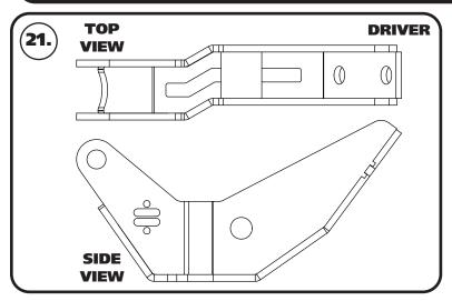
**21.** The lower shock mount offsets the bottom of the shock to the wheel for better spring clearance. The Driver lower shock mount is shown in **Image 21**.
