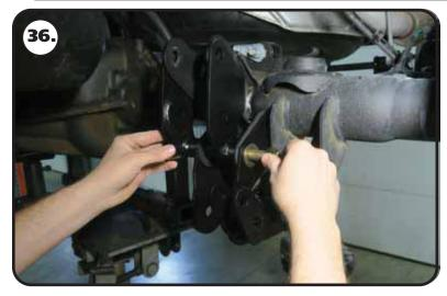
**36.** Install a M16 flat washer and M16-2.0 nylok nut on the threads of the bolt. Do not tighten this hardware at this time.
