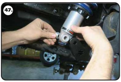
**47.** Insert the shock bearing spacers into the bearings of the bearings of the coilover. The small diameter of the spacers will get inserted into the bearing.
