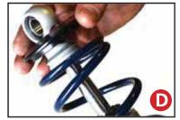
Once the knob is removed slide a Delrin washer over the eyelet. Next, slide the upper spring mount (803-00-199) over eyelet as seen in figure D.
