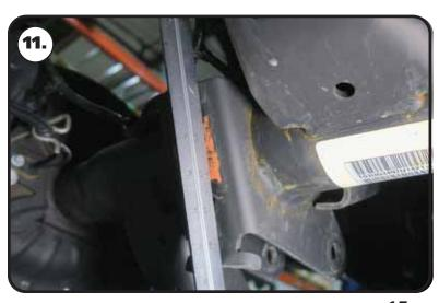
**11.** The rear surface of the control arm/sway bar mount needs to be flat. The lower edge is bent, but will need to be flattened. Use a straight edge to see how much it needs to be flattened.
