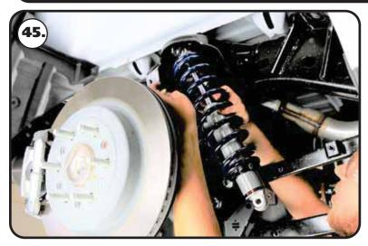
**45.** Insert the eyelet of the coilover in the previously installed upper shock mount. Line up the through hole of the bearing/spacers with the mounting holes of the upper shock mount.
