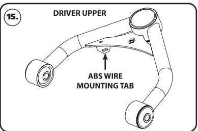
**15.** The upper control arms are side specific. The driver control arm is shown in **Image 15**. The ABS wire tab is to the rear of the truck.
