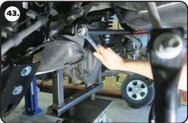
**43.** Insert the other end of the panhard in the mount on the axle. Insert the OEM panhard hardware and install the nut. Do not tighten the hardware at this time. The hardware will be torqued after the truck is on the ground.
