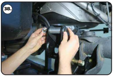
**38.** Install a M16 flat washer on a M16-2.0 x 120mm bolt. Insert the bolt through the aligned holes. Install a M16 flat washer & M16-2.0 nylok nut on the threads of the bolt. Do not tighten hardware at this time.
