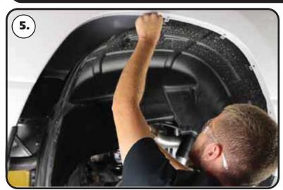
5. Remove the rear wheel liners. Retain the liners and the hardware to reinstall them after the lowering kit has been installed.
