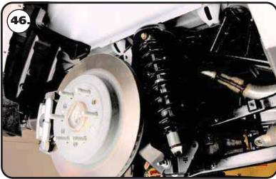
**46.** Install a 1/2" flat washer on a 1/2"-13 x 2 3/4" bolt. Insert the bolt/washer into the upper mount/shock. Install a 1/2" flat washer and 1/2"-13 nylok nut and Torque to 75 ftlbs.
