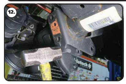
**12.** Use a hammer to flatten the bottom of the control arm/sway bar mount.
