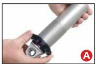
First, using the supplied lower adjuster nut (803-00-199) thread the nut onto the shock from the bottom side as seen in figure A. Remove the plastic pellet that is in the split of the adjuster nut.
