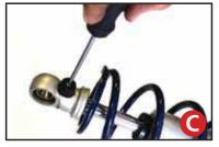
Before the upper spring mount can be installed screw the adjuster knob on the upper eye mount to the firmest setting (clockwise) as seen in figure C. Then remove the Knob by holding it while removing the center screw.
