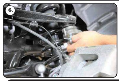
**6.** The upper control arm will need to be disconnected from the steering knuckle. Remove the OEM upper control arm. Retain the hardware to install the new upper control arm.
