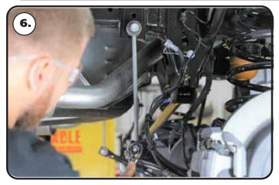
**6.** Remove the sway bar linkage. It will be replaced with new linkage.
