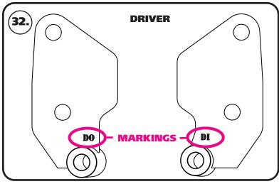
**32.** This kit requires the upper control arm to be relocated to correct the geometry for the new ride. The kit includes brackets for relocating the upper control arms. The control arm brackets are marked for vehicle side and location. **Image 32** illustrates the driver side relocation brackets. They are marked DO for Driver Outer and DI for Driver Inner. The flat side of the bracket is positioned to the front of the truck.
