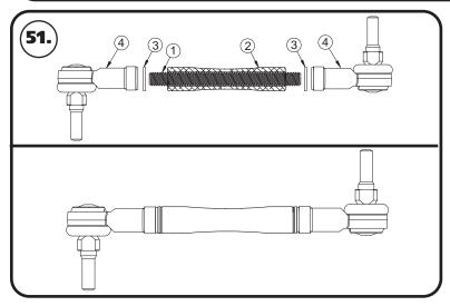
**51.** The sway bar linkage will need to be assembled. Insert the M10-1.5 x 130mm threaded stud in the 3.68" spacer. Put a copper crush washer on each end of the threaded stud. Put red loctite on the threads of each end of the stud. Thread a 90 degree end on each end and tighten the ends. The studs need to be pointing away from each other after the linkage is tight. See **Image 51**.
