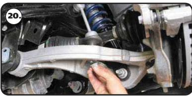
**20.** Reattach the sway bar linkage. The lower sway bar linkage nut is torqued to 75 ft-lbs.
