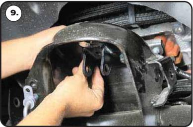
**9.** Position the upper coil over mount in the OEM location with the flat side positioned to the frame. Install a M12 flat washer on each of (3) M12-1.75 x 30mm hex bolts. With the mounting holes aligned, insert a bolt/washer in each hole. Install a M12 flat washer & M12-1.75 nylok nut on each bolt. Torque the bolts to 69 ft-lbs.
