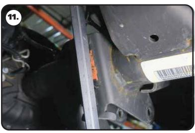
**11.** The rear surface of the control arm/sway bar mount needs to be flat. The lower edge is bent, but will need to be flattened. Use a straight edge to see how much it needs to be flattened.
