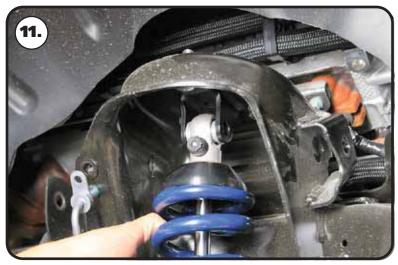
11. Insert the shock eyelet into the upper mount. Install each CoilOver in the upper mount with the Adjusting Knob facing the wheel of the truck. Line up the shock bearing/spacers hole with the mounting holes of the upper mount.
