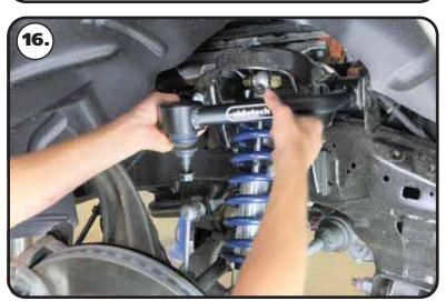
**16.** Install the Ridetech upper control arms using the OEM hardware. The control arms are mounted in the OEM mounts with the ABS wire tab to the rear of the truck. The control arm mounting bolts will need to be tightened after the truck is sitting on the ground.
