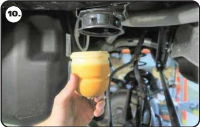
**10.** The OEM bump stop mount will need to be removed. The bump stop snaps into the OEM mount. Push on the side of it to get it to pop out of the mount.
