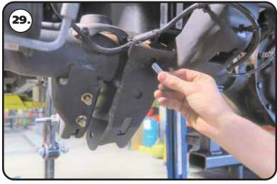
**29.** Install a M10 flat washer on a M10-1.5 x 30mm bolt. Install the bolt/washer in one of the rear holes. Snug the bolt down, but do not torque since it will be removed later.
