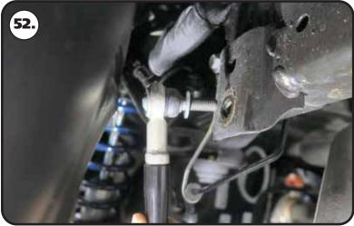
**52.** Install a M10 flat washer on the threaded stud of sway bar linkage. Apply red loctite to the threads of the end link and thread it into the OEM sway bar linkage mount.
