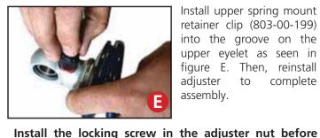
Install upper spring mount retainer clip (803-00-199) into the groove on the upper eyelet as seen in figure E. Then, reinstall complete adjuster to assembly.
