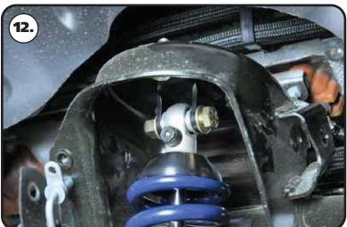
**12.** Install a 1/2" flat washer on a 1/2"-13 x 2 1/2" bolt. Insert a bolt/washer through the mount/shock. Install a 1/2" flat washer and 1/2"-13 nylok nut on the threads of the bolt that are sticking through the mount. Torque the upper mounting hardware to 75 ftlbs.
