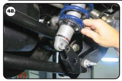
**48.** Insert the body of the coilover in the previously installed lower shock mount. Line up the through hole of the bearing/spacers with the mounting holes of the lower shock mount.
