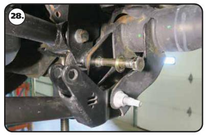
**28.** Align the OEM lower bar mounting hole with the hole in the new mount. Insert a M16-2.0 x 170mm bolt through the hole to keep it aligned. Do not put a nut on the bolt as it will be removed later.
