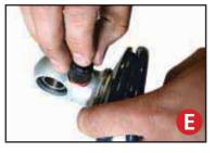
Install upper spring mount retainer clip (038-01-006-A) into the groove on the upper eyelet as seen in figure E. Then, reinstall adjuster to complete assembly.
