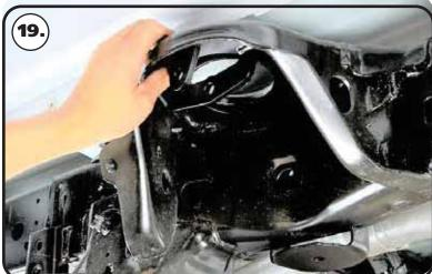
**19.** Align the upper shock mount with the holes in the OEM coil spring mount. Again, the Arrow will point to the front of the truck with the shock mount out away from the frame.
