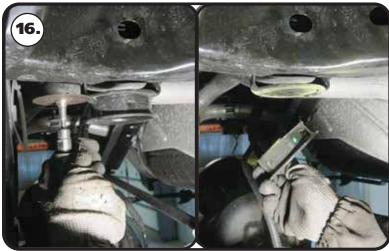
**16.** The bump stop mounting ring will need to be cutoff the truck. Just the ring needs cutoff, leaving the mount the ring is welded to. It can be cut off with a die grinder and cutoff wheel by cutting the welds. Grind the surface smooth and paint it.
