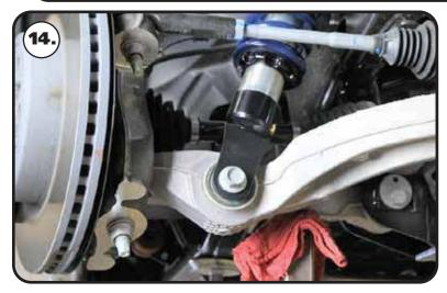
**14.** Install the OEM lower shock bolt. We recommend installing the bolt with the threads to the rear of the truck. Instal the OEM nut on the threads of the bolt. Torque the shock bolt to 125 ft-lbs.
