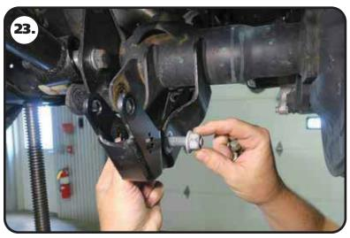
**23.** Install the OEM nut on the OEM bolt, but do not tighten until the (2) rear bolts are installed.
