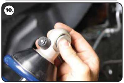
**10.** Install the 1/2" I.D. bearing spacers into the bearing in the shock eyelet. These spacers have a through hole that is 1/2" diameter. The small diameter of the spacers will insert into the shock bearing.
