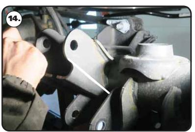
**14.** The front of the OEM upper bar mounts will need to be cutoff. Images 14 & 15 show the mount marked and after it has been cut. Mark a straight line from where the end radius stops to just where the weld on the axle tube stops
