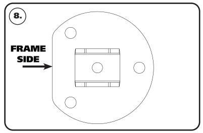
**8. Image 8** illustrates the upper coil over mount. The flat side of the mount will need to be positioned to the frame.
