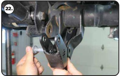
**22.** The lower shock mount will be positioned in the OEM lower shock mount. The large mounting hole will align with OEM shock mounting hole. Align the holes and insert the OEM shock bolt in the aligned holes.
