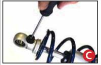
Before the upper spring mount can be installed screw the adjuster knob on the upper eye mount to the firmest setting (clockwise) as seen in figure C. Then remove the Knob by holding it while removing the center screw.
