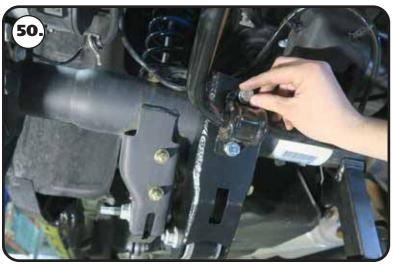
**50.** Install a M10 flat washer on each of (4) M10-1.5 x 30mm hex bolts. Hold the OEM sway bar in position and attach it using the (4) bolts/washer in the OEM mounting holes. Do not tighten the hardware until the sway bar linkage is installed.
