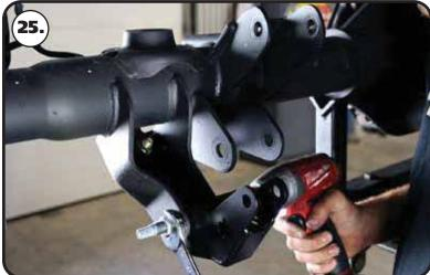
25. Torque the OEM shock bolt to 100 ft-lbs.
