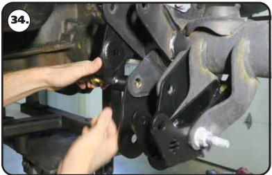
**34.** The upper brackets need to be installed to relocate the upper bars. Each bracket will be positioned to the outside of the OEM upper bar mount. Start by aligning the sleeve on the Inner bracket with the OEM lower bar mounting hole. Install a M16 flat washer on a M16-2.0 x 170mm bolt. Insert the bolt through the sleeve and through the OEM lower bar mounting hole. Make sure the bolt is not sticking through the OEM mount. If it is sticking out, the outer bracket can not be inserted.
