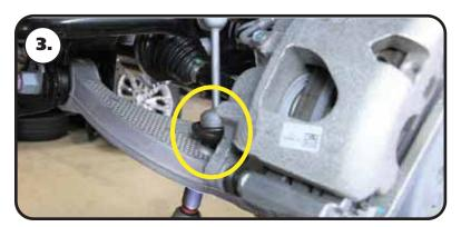
**3.** Disconnect the sway bar from the control arms. This allows the lower control arm to move easier during the CoilOver installation.
