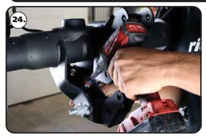
**24.** Install a 3/8" flat washer on each of (2) 3/8"-16 x 1 1/4" hex bolt. Insert the bolts/ washers in from the bottom. Install a 3/8" flat washer & 3/8"-16 nylok nut on each bolt. Torque the 3/8" hardware to 35 ft-lbs.
