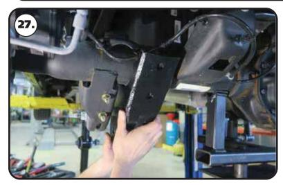
**27.** The lower relocation bracket will slip over the OEM lower bar bracket.
