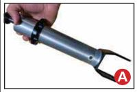
First, using the supplied lower adjuster nut (234-15-200) thread the nut onto the shock from the top of shock as seen in figure A. Remove the plastic pellet that is in the split of the adjuster nut.
