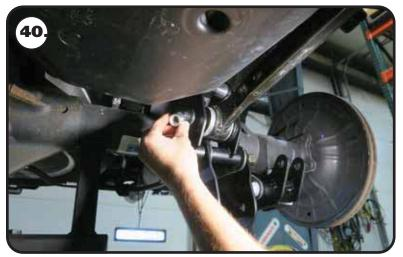
**40.** Align the end of the upper bar with the center holes of the relocation brackets. Install a M16 flat washer on a M16-2.0 x 120mm bolt. Insert the bolt through the aligned holes.
