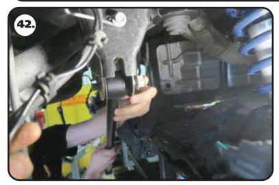
**42.** Both ends of the new panhard bar are the same. Insert one end of the panhard in the OEM frame mount. Insert the OEM panhard hardware and install the nut. Do not tighten the hardware at this time.
