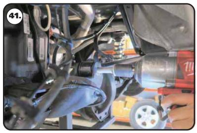
**41.** Remove the OEM panhard bar. Retain the OEM hardware for installation of the new panhard bar.
