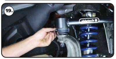
**19.** Insert the OEM ABS clip into the tab of the control arm.
