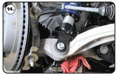
**14.** Install the OEM lower shock bolt. We recommend installing the bolt with the threads to the rear of the truck. Instal the OEM nut on the threads of the bolt. Torque the shock bolt to 125 ft-lbs.
