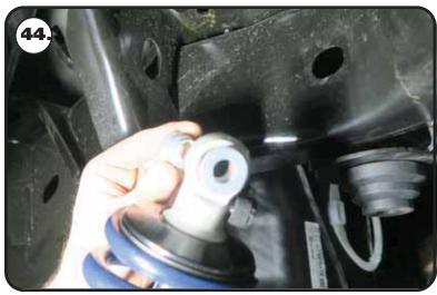
**44.** Insert the shock bearing spacers into the bearings of the eyelet of the coilover. The small diameter of the spacers will get inserted into the bearing.
