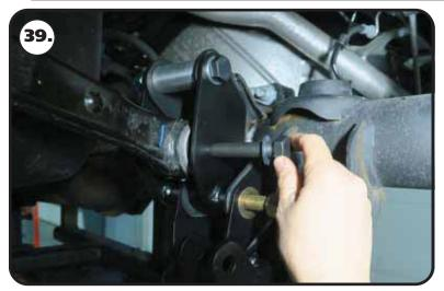
**39.** Align the end of the upper bar with the center holes of the relocation brackets. Install a M16 flat washer on a M16-2.0 x 120mm bolt. Insert the bolt through the aligned holes.
