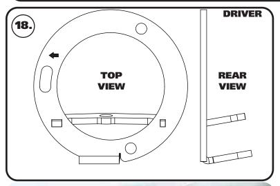
**18.** The upper shock mounts are side specific. **Image 18** shows the Driver side upper mount. The arrow that is cut in the bracket will point to the front of the truck with the coilover moved out away from the frame.
