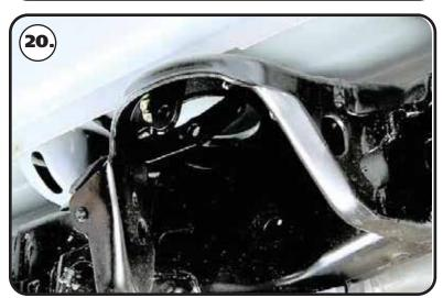
**20.** Install a 3/8" flat washer on each of (3) 3/8"-16 x 1 1/4" bolts. Hold the bracket in position and put the bolts/washer through the mounting holes. Install a 3/8" flat washer & 3/8"-16 nylok nut on each of the bolts. Torque hardware to 35 ft-lbs.
