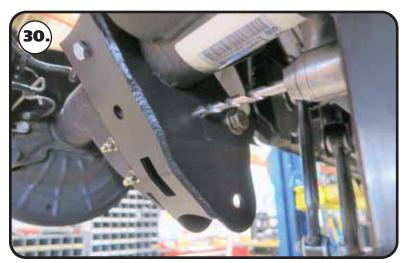
**30.** There is a hole on the inside of the bracket that will need to be used as a template to drill a 3/8" hole in the OEM mount. Drill the hole with a 3/8" drill bit. Install a 3/8" flat washer on a 3/8"-16 x 1 1/4" bolt. Insert the bolt/washer in the drilled hole. Install a 3/8" flat washer & 3/8"-16 nylok nut on the bolt. Torque the hardware to 35 ft-lbs.
