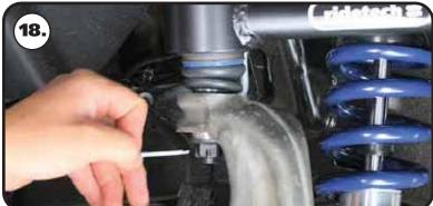
**18.** Install the supplied cotter pin. Bend the tabs of the cotter pin.
