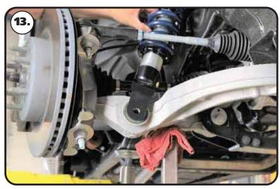
**13.** Use a jack under the lower control arm to raise the control arm. Align the OEM shock mount with the lower shock mount of the coil over.
