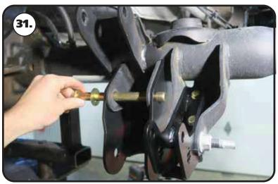
**31.** Remove the M16-2.0 x 170mm bolt from the lower mount.
