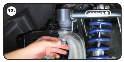
17. Insert the ball joint stud into the spindle. Install (2) M14 flat washers on the ball joint stud. Next, install the ball joint nut and torque to 50 ft-lbs. Tighten the nut until a slot in the nut aligns with the hole in the ball joint pin. NEVER LOOSEN THE NUT TO ALIGN THE HOLE!
