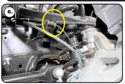
**6.** Disconnect the ABS wire and clip from the OEM control arm. The clip will be reused with the new control arms.
