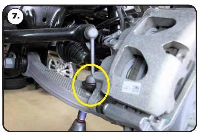
**7.** Install the Ridetech upper control arms using the OEM hardware. The control arms are mounted in the OEM mounts with the ABS wire tab to the rear of the truck. The control arm mounting bolts will need to be tightened after the truck is sitting on the ground.
