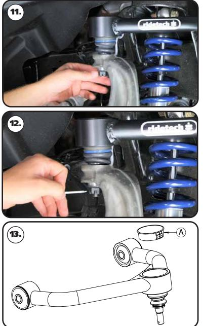
**11.** Insert the ball joint stud into the spindle. Install (2) M14 flat washers on the ball joint stud. Next, install the ball joint nut and torque to 50 ft-lbs. Tighten the nut until a slot in the nut aligns with the hole in the ball joint pin. NEVER LOOSEN THE NUT TO ALIGN THE HOLE!
