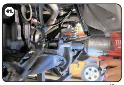
**41.** Remove the OEM panhard bar. Retain the OEM hardware for installation of the new panhard bar.
