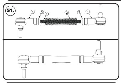
**51.** The sway bar linkage will need to be assembled. Insert the M10-1.5 x 130mm threaded stud in the 3.68" spacer. Put a copper crush washer on each end of the threaded stud. Put red loctite on the threads of each end of the stud. Thread a 90 degree end on each end and tighten the ends. The studs need to be pointing away from each other after the linkage is tight. See **Image 51**.
