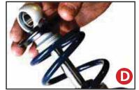
Once the knob is removed slide a Delrin washer over the eyelet. Next, slide the upper spring mount (803-00-199) over eyelet as seen in figure D.
