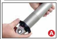
First, using the supplied lower adjuster nut (803-00-199) thread the nut onto the shock from the bottom side as seen in figure A. Remove the plastic pellet that is in the split of the adjuster nut.
