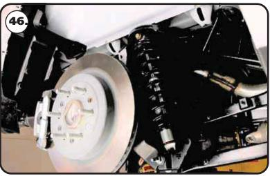
**46.** Install a 1/2" flat washer on a 1/2"-13 x 2 3/4" bolt. Insert the bolt/washer into the upper mount/shock. Install a 1/2" flat washer and 1/2"-13 nylok nut and Torque to 75 ftlbs.
