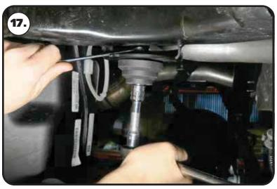
**17.** Bolt the supplied bump stops to the flat surface of the OEM mount. It is attached using (1) 3/8"-16 x 1" socket head cap screw, (1) 3/8" SAE flat washer, & (1) 3/8"-16 nylok nut. Torque to 35 in-lbs.
