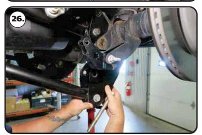
**26.** The lower bar bracket is the same for driver and passenger. The lower bar will need to be inserted into the bracket before putting it in place. The bolt must be installed from the outside with the threads pointing in. This reuses the OEM lower bolt. The bar mounting bolt needs to be left loose.
