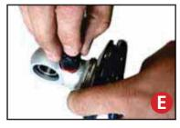
Install upper spring mount retainer clip (803-00-199) into the groove on the upper eyelet as seen in figure E. Then, reinstall adjuster to complete assembly.
