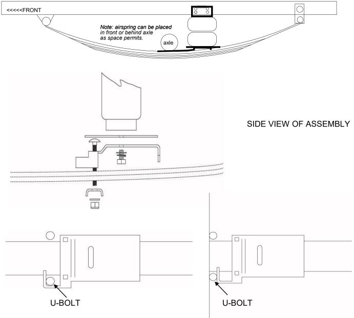
THE LEAF SPRING BRACKET CAN BE INSTALLED HOOKED ON THE U-BOLT OR TOUCHING U-BOLT AS SEEN IN ABOVE ILLUSTRATIONS.
