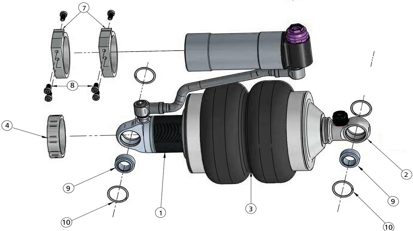
**WARNING: ATTEMPTING TO REMOVE THE AIR FITTING WILL DAMAGE IT AND VOID THE WARRANTY.**
