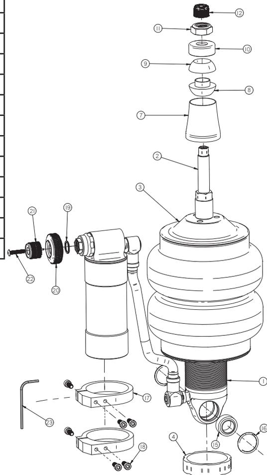
**THE DELRIN BALL REQUIRES A 3/4" HOLE FOR THE FLANGE TO GO THROUGH. THIS CAN BE DRILLED WITH A UNIBIT.**
