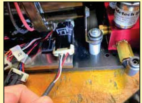
Run the harness from the sensors to the Main Harness (AirPod). We recommend marking the harnesses at the end that will plug in at the Main Harness (AirPod). The 4 plugs in the Main Harness are labelled for each corner. Plug the correct harness into each plug.
