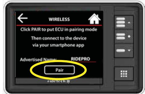
**Step 2:** Go to the Wireless tab under the Menu on the control panel and select it. You should see the screen above. Touch the pair button on the control panel.
