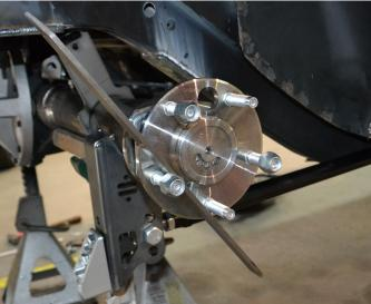
This picture shows the mount on the rearend with the bar in the correct center hole.
