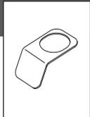
1 Secure the heat shield by clamping it between the air spring and upper spring mount assembly.
