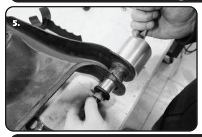
**5.** Slide the Aluminum Spacer Sleeve onto the Threaded Rod followed by the Pushing Washer, Flat Washer and Hex Nut. Run the nut down snug, making sure the 2.625" washer is centered on the 2.375" Sleeve. Using wrenches, tighten the Hex Nut to push the bushing out of the control arm.
