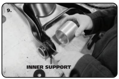
**9.** The 2.375" Sleeve/2.625" Washer will be placed against the control on the inner side that the bushing will be pushed into. **IT IS VERY IMPORTANT THAT THE NO EDGE OF THE 2.375" SLEEVE GETS OVER THE BUSHING HOLE, IN THE CONTROL ARM, WHILE INSTALLING THE BUSHING SHELL. This can cause the bushing shell to crash into the bushing as you are installing it. Insert the 1/2"-10 x 8" Threaded Rod into the 2.625" Washer and through the bushing sleeve.**
