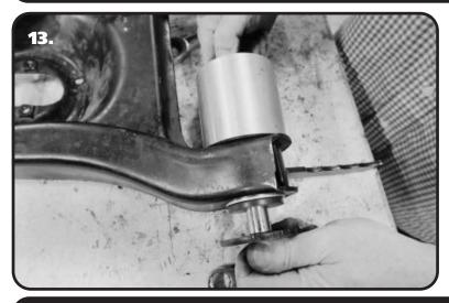
**13.** Use the 2.375" Sleeve, 2.625" Washer, 1/2" Threaded Rod, Large Washer, 1/2" Flat Washer, 1/2" Hex Nut, used to push the shell into the arm, to finish pushing the inner sleeve into the delrin bushing. Tighten the nut until the sleeve is all the way in the bushing.
