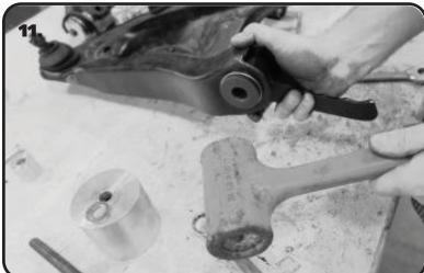
**11.** Start the correct delrin bushing into the shell by hand. Tap it the rest of the way in with a hammer. The assembly used to push the shell in can also be used. Bottom the bushing flange against the flange of the shell.
