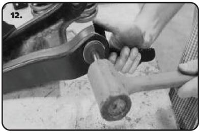
**12.** Start the correct inner sleeve into the delrin bushing. You can tap it in some with a hammer. Be careful to not distort the edge of the bushing with the hammer.
