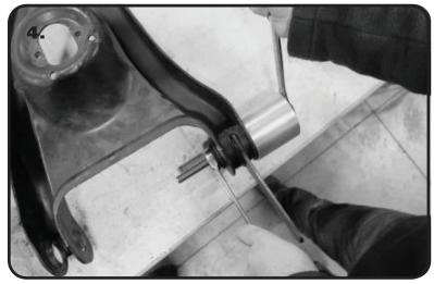
**4.** Using a wrench on each hex, tighten the nut. The bushing should start pushing out of the arm. Tighten the nut, pushing the bushing out, until the washer is just through the inner surface of the control arm. Loosen the nut, removing the nut/ flatwasher and pushing washer.
