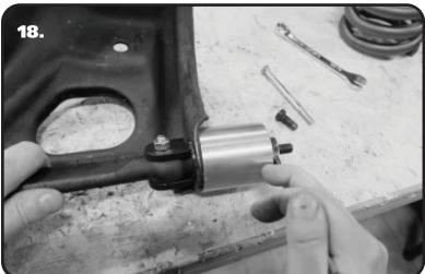
**18.** Tighten the 3/8"-24 Nut down, pushing the bushing out of the control arm. It may be necessary to loosen the assembly and turn the cross shaft in the bushing if the bushing would happen to start pushing out crooked. Tighten the nut until the tabs bottom out or push the bushing out. If the tabs bottom out before the bushing is completely out, you should be able to tap it out with a hammer.
