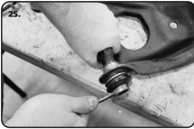
**25.** With all of the bushings and cross shafts installed, install the OEM hardware and tighten it down pushing the bushings in the remainder of the way.
