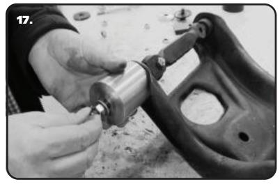
17. Insert the 3/8"-24 x 3" threaded rod into the 2.625" OD washer. Position the 2.25" Sleeve over the bushing. Insert the threaded rod/washer setup through the 2.25" sleeve threading the rod into the end of the cross shaft. Thread it in until it stops. Install a 3/8" Flatwasher onto the threaded rod followed by a 3/8"-24 Hex nut. Thread the nut down until all parts are snug. Be sure the 2.25" sleeve is around the flange of the bushing and not on top of it anywhere.
