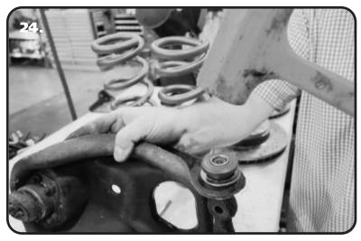
**24.** Lightly tap the bushing/sleeve into the bushing shell. There will probably be a little gap left. The OEM Hardware will be used to push the bushings in the remainder of the way.
