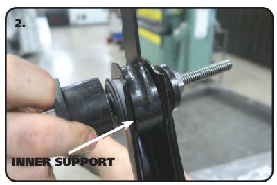
**2.** Start by sticking the Inner Arm Support in the arm with the "C" shape cradling the bushing. This support keeps the control arm from deforming while removing and installing the bushings.
