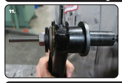
**11.** Use the 1.875" Sleeve, 2.125" Washer, 1/2" Threaded Rod, Large Washer, 1/2" Flat Washer, 1/2" Hex Nut, used to push the shell into the arm, to finish pushing the inner sleeve into the delrin bushing. Tighten the nut until the sleeve is all the way in the bushing. Remove the tool. Install the Delrin Spacer, use **Image 8** as a reference.
