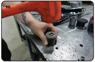
**10.** Install the correct inner sleeve into the delrin bushing. You can tap it in with a hammer. Be careful to not distort the edge of the bushing with the hammer. Once the Inner Sleeve is installed, start the assembly into the outer shell installed in the arm. It can be pushed partially in by hand,
