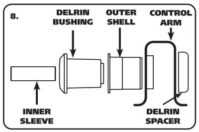
**8. Image 8** is a exploded view of the lower control arm bushing. These Bushings use a Delrin Spacer on one side of the control arm. **The Spacer goes on the opposite side of the bushing flange.** With the Delrin Bushing and Inner Sleeve installed, install the Delrin Spacer over the SMALL end of the Delrin Bushing. The ROUNDED surface will be out, away from the control arm.
