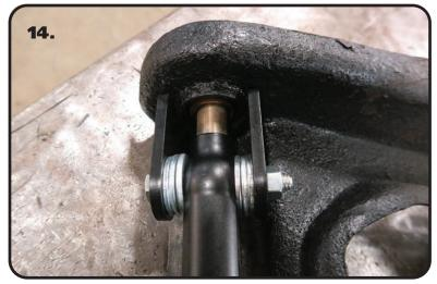
**14.** Bolt the Short Cross Shaft Tabs to the cross shaft using (1) 5/16"-18 x 2 1/4" Hex Bolt, (6) 3/8" Flat Washers & (1) 5/16" Hex Nut. The Tabs will be bolted to the cross shaft using the cross shaft mounting holes with (3) 3/8" Flat Washers between each Tab and The Cross Shaft. Place a Tab on each side of the cross shaft with the flat side against the control arm. Tighten the 5/16" bolt/nut with the flats squarely against the control arm.
