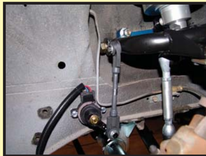
5- Once both sides of the linkage have been finished, secure the linkage to the sensor and suspension.
