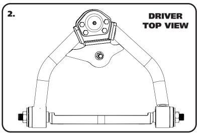
**2.** The Upper Control Arm is attaching the factory mount using factory hardware. The driver side arm is shown in **Figure "2"**. The Ball Joint located on the arm to the rear of the car.
