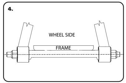
**4.** Attach the Upper Control Arm with the FLAT Side of the cross shaft against the frame. Attach the upper control arms using the OEM hardware.
