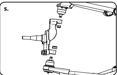
**5.** Attach the Spindle to the control arms. The Spindle is the same for Driver and Passenger.
